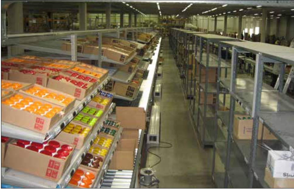
Flow racks and conveyor system
